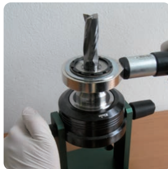
Tighten the nut using the torque wrench
