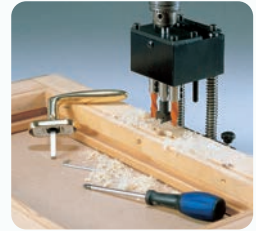
DRILLING JIG FOR CREMONE BOLTS Page 16.07
