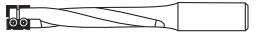
HW INSERT ROUTER BITS FOR LOCKS Z=2 HEAVY METAL TOOL BODY Page 9.14
